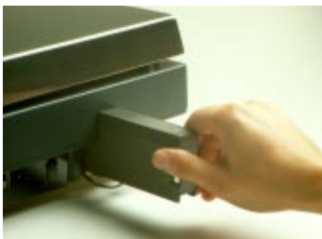
Quick Count is portable when equipped with an optional internal camcorder battery.
